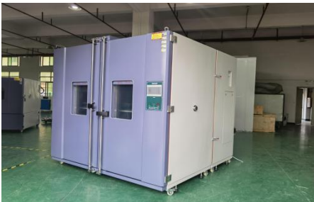
3.6 m3 constant temperature humidity laboratory
