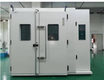
3.6 m3 constant temperature humidity laboratory
